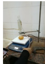
Adding the catalyzed alcohol to oil and keep stirring for 2 hours at 130 °C
