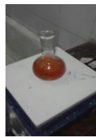
Heating the oil at 130 °C
